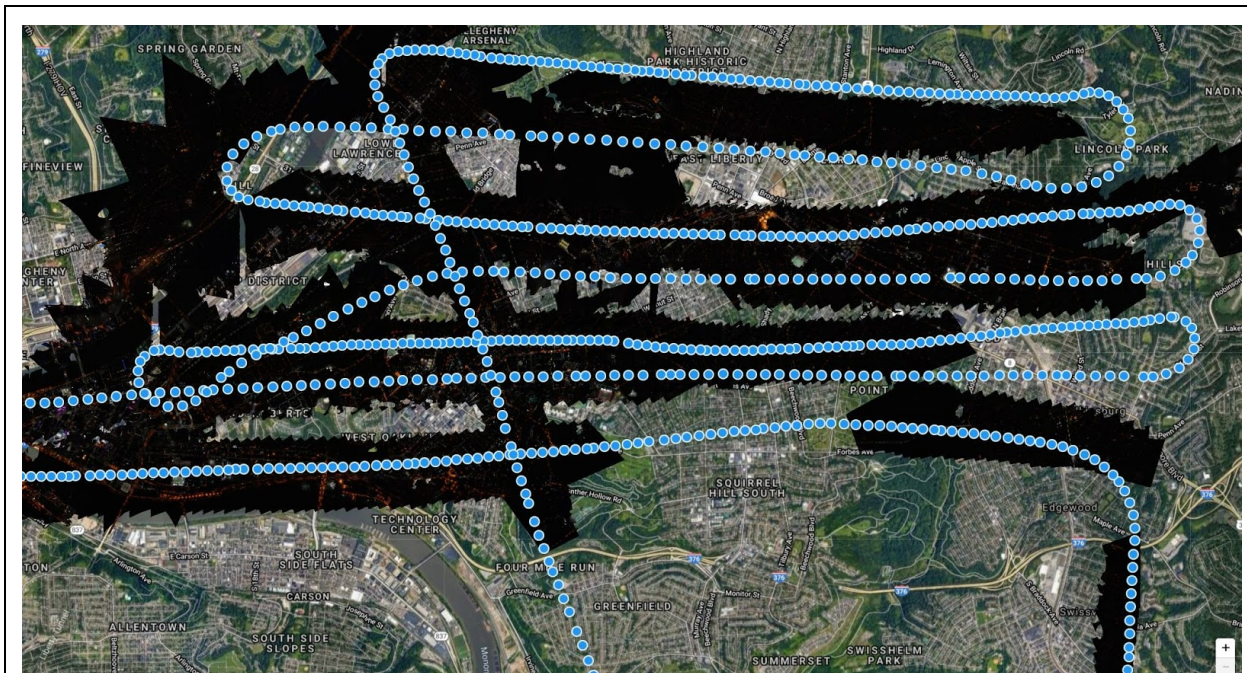
Fig. 4 DroneDeploy map generated from using python processed imageset. The blue dots represent geolocation of photos used for rendering.
